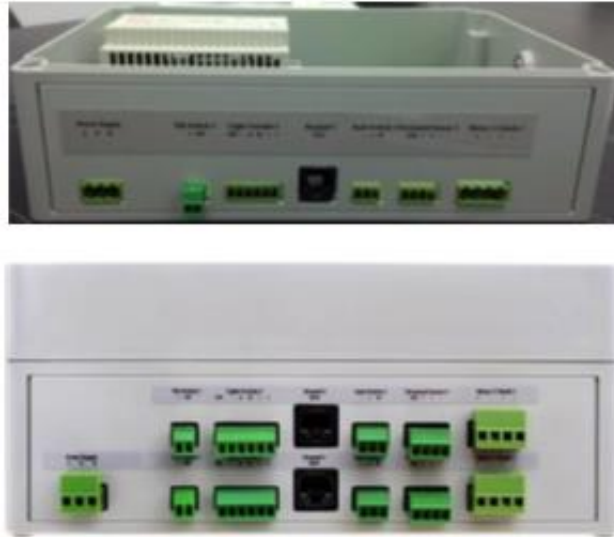
Figure 30: Auto Sash Control Unit Connectors, Single and Dual Fume Hoods
